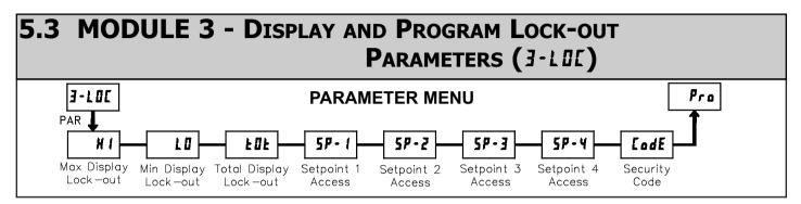
Module 3 is the programming for Display lock-out and "Full" and "Quick" Program lock-out.
